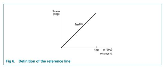
The angular range is set to  $\alpha_{max}$  = 180° and the clamping voltages are programmed to  $V_{(CL)l}$  = 5 % $V_{DD}$  and  $V_{(CL)u}$  = 95 % $V_{DD}$  for a valid definition of errors.
