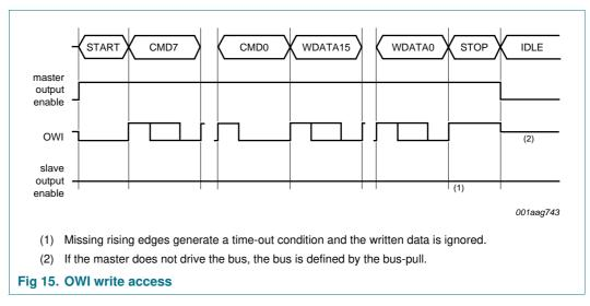
**Note**: As already mentioned in Section 13.1, the command mode has to be entered using the write procedure. If command mode is not entered, communication is not possible and the sensor operates in normal operation mode. After changing an address, the time  $t_{prog}$  must elapse before changing another address. Finally the checksum must be recalculated and written, because the contents of the non-volatile memory have been changed (see Section 13.4).
