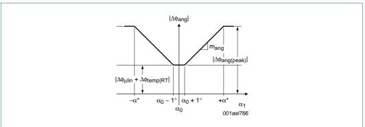
Fig 11. Envelope curve for the magnitude of angular error
