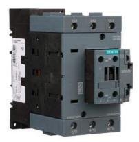
Electrically held lighting contactor, Contactor amp rating 100A, 0 N.C. / 3 N.O. Poles, 600VAC 60HZ coil, 1 NO / 1 NC auxiliary contacts Non-combination type, (no disconnect device), Enclosure NEMA type (open), No enclosure
