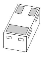
PBSS3515M 15 V, 0.5 A PNP low V<sub>CEsat</sub> (BISS) transistor
