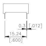
NOTES: All dimensions are in millimeters. Tolerances are ± 0.25 mm (0.01") unless otherwise noted.
