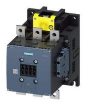
Power contactor, AC-3 225 A, 110 kW / 400 V Coil AC 50/60 Hz and DC 96-127 V x (0.8-1.1) F-PLC input 24 V DC 3-pole size S10 Auxiliary contacts 2 NO + 2 NC Main circuit: Busbar Control and auxiliary circuit: screw terminal
