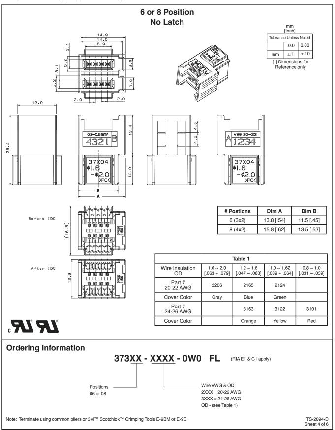
Designed for Wiring Supplied from Japan and Asia, 2 mm, IDC, Wiremount, Panel Mount 373 Series
