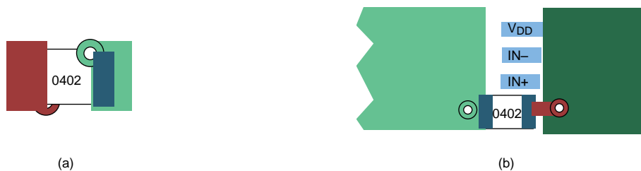
Figure 27. Typical Decoupling Capacitor Layouts
