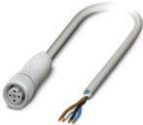
Sensor/Actuator cable, 4-position, PP-EPDM halogen-free, Gray RAL 7035. Free cable end, on Socket straight M12, A-coded, Cable length: 1.5 m, Hygienic design, with plastic knurl
