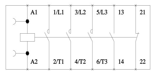
LEN00C003 Wiring Diagram
