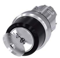
RONIS key-operated switch, 22 mm, round, metal, shiny, lock number 455, with 2 keys, 2 switch positions O-I, latching, actuating angle 90°, 10:30h/13:30h, key removal O+I, with laser labeling, inscription or symbol Customer-specific selection with SIRIUS ACT configurator (CIN)
