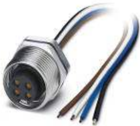
Sensor/actuator flush-type socket, 4-pos., 7/8", rear mounting with M26 fastening thread, with 1.0 m PE litz wire, 4 x 0.75 mm 2
