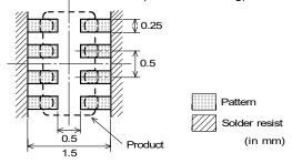
\* The excessive heat by land pads may cause deterioration at joint of products with substrate.
