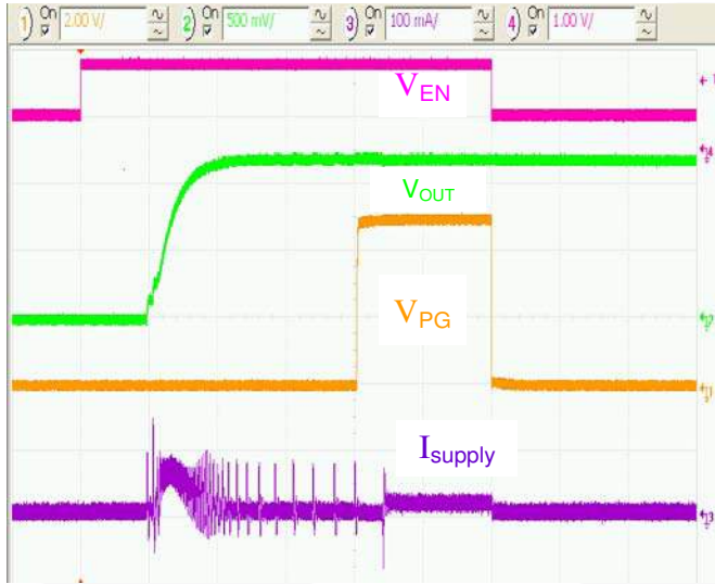
Figure 15. Soft-Start: EN Voltage Raised After V_{IN} = 5.0\text{ V} , I_{LOAD} = 0 , Horizontal Scale = 100\ \mu\text{s}/\text{div} .
