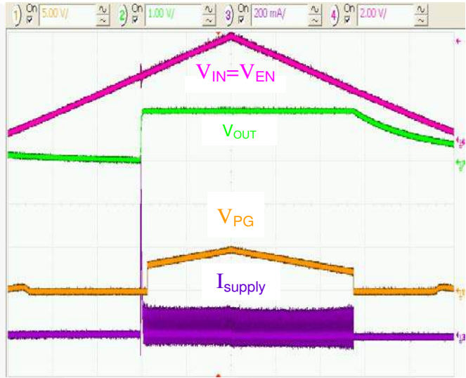
Figure 16. Soft-Start: EN Pin Tied to VCC, I_{LOAD} = 0 , Horizontal Scale = 1\text{ ms}/\text{div} .
