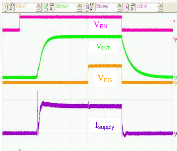
Figure 17. Soft-Start: EN Pin Raised after V_{IN} = 5.0\text{ V} , R_{LOAD} = 400\text{ m}\Omega , C_{OUT} = 100\ \mu\text{F} , Horizontal Scale = 100\ \mu\text{s}/\text{div} .
