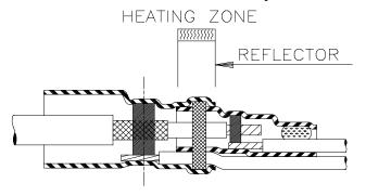
Position the center sealing insert of the SolderSleeve termination assembly whithin the heating tool reflector and apply heat until soldersleeve tubing collapses onto cable dielectric. Move assembly whithin the reflector to the large solder preform and apply heat until it melts and flows forming a solder fillet between the cable shield and the ground wire and then shrink the tubing onto the cable jacket.
