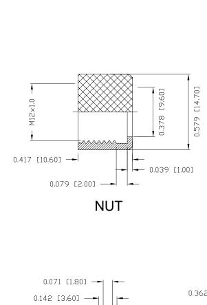
DESCRIPTION: M12 FEMALE - CABLE MOUNT - SOLDER CUP - 4 POS. - D CODE
