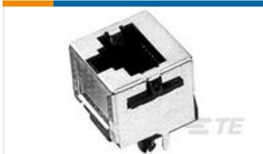
TE Part #2-1734858-3 RJ11,8P8C,TOP ENTRY,SMT,30u"
