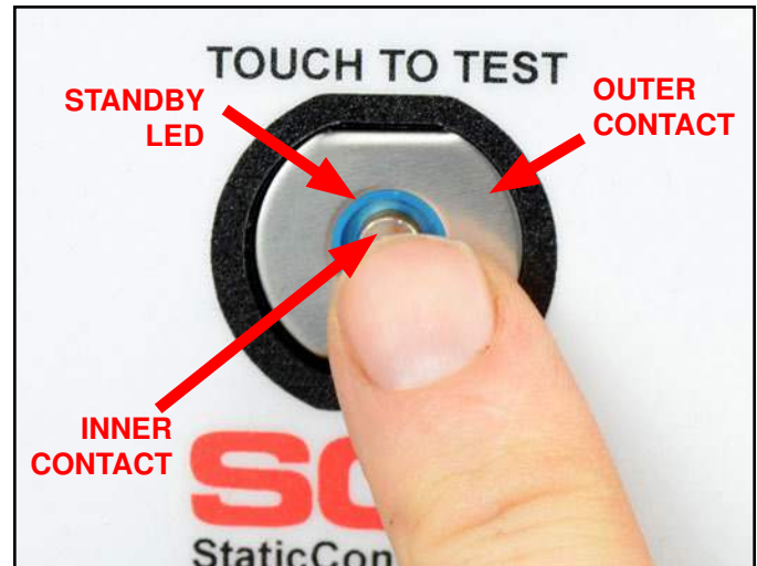
Figure 9. Steady-State Test Switch features and components
