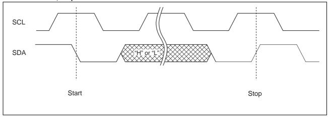
Note: At the write operation, the FRAM device does not need the memory programming wait time (twc) after issuing the Stop Condition.
