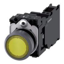
Illuminated pushbutton, 22 mm, round, plastic with metal front ring, yellow, pushbutton, flat, momentary contact type, with holder, 1 NO+1 NC, LED module with integrated LED 24 V AC/DC, Spring-type terminal
