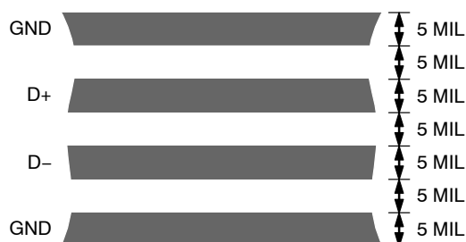
Figure 16. Arrangement of Signal Tracks
