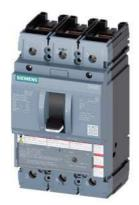
circuit breaker 3VA5 UL frame 250 breaking capacity class H 65kA @ 480 V 3-pole, line protection TM230, FTAM, In=100A overload protection Ir=100A fixed short-circuit protection Ii=5...10 x In cable connection on both sides
