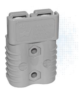
The SB<sup>®</sup> 2/0 is an extension of the SB<sup>®</sup>175 connector series with more power in the same footprint. The SB<sup>®</sup> 2/0 features outer dimensions that are identical to the SB<sup>®</sup>175, but has been designed to accept only a contact for 2/0 or 70mm<sup>2</sup> wire.
