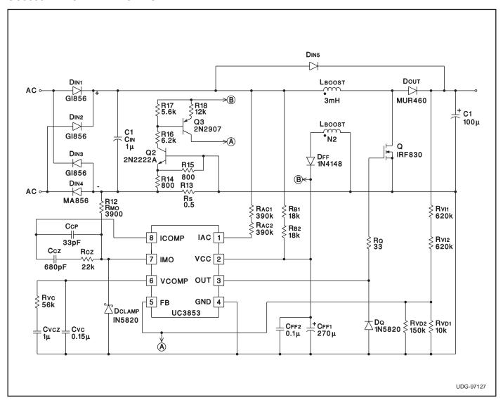
Note: the application circuit shown is a 100W, 75KHz design. Additional application information can be found in Application Note U–159 and Design Note DN–78.
