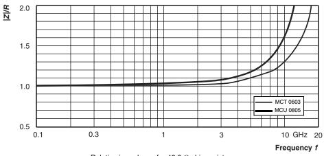
Relative impedance for 49.9  $\Omega$  chip resistor
