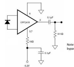
Note that the 10W resistor and bypass capacitor are critical.
