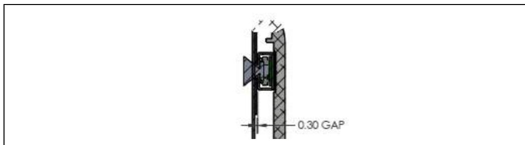
Figure 7-13. Stereo Depth Module Air Gap
