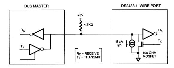
The idle state for the 1 wire bus is high. If for any reason a transaction needs to be suspended, the bus MUST be left in the idle state if the transaction is to resume. Infinite recovery time can occur between bits so long as the 1-Wire bus is in the inactive (high) state during the recovery period. If this does not occur and the bus is left low, all components on the bus will be reset. See Wire-1 Reset Pulse Timing (Figure 9).
