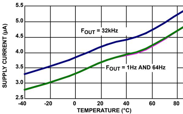
FIGURE 9.  $I_{DD}$  vs TEMPERATURE, 3 DIFFERENT  $F_{OUT}$
