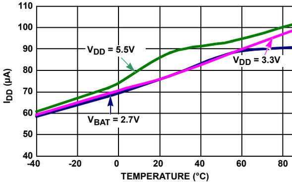
FIGURE 11.  $I_{DD}$  with TSE = 1 vs TEMPERATURE
