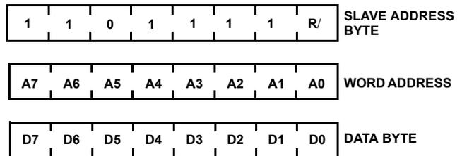
FIGURE 19. SLAVE ADDRESS, WORD ADDRESS AND DATA BYTES
