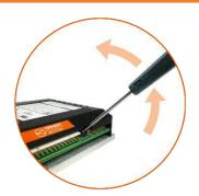
To turn off a switch, use a tool such as a small screwdriver to gently pull the switch backward. *Tip: use the underside of the cover as a fulcrum and the screwdriver as a lever to pull the switch backward*
