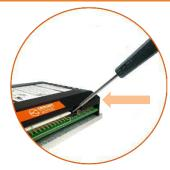
To turn on a switch, use a tool such as a small screwdriver to gently push the switch forward
