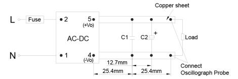
C1:Ceramic capacitor,1uF; C2:Electrolytic capacitor,10uF
