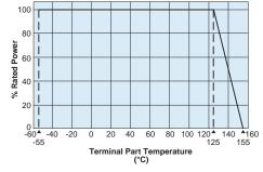
For resistors operated at a terminal part temperature of described for each size or above, a power rating shall be derated in accordance with the above derating curve. Please refer to "Introduction of the derating curve based on the terminal part temperature" in the beginning of our catalog before use.
