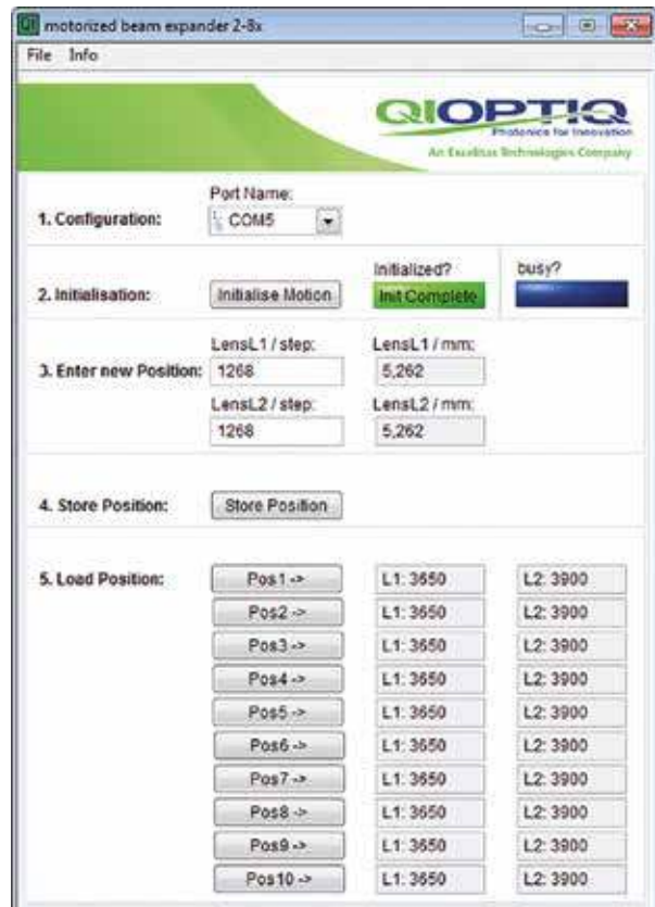
Windows™ software mask for easy control of motorized Beam Expanders.
