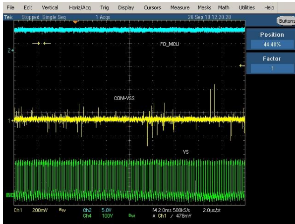
Figure 31. During startup, current is high, with shorted COM-VSS, noise is less, fault conditions do not occur, compressor will not stall, 2ms/div
