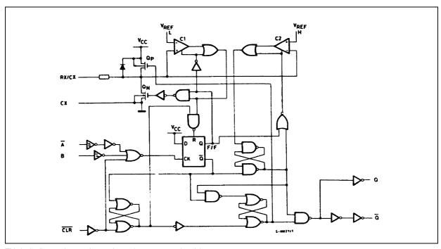
This logic diagram has not be used to estimate propagation delays
