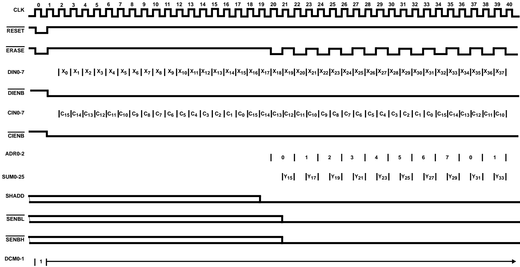
FIGURE 7. 16-TAP DECIMATE-BY-TWO FIR FILTER TIMING; 30MHz, 15MHz OUT
