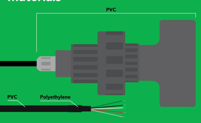
Connecting this probe to these devices will give you a sensing range of:
