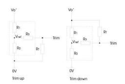
Application circuit for TRIM (Part in broken line is the interior of models) Note: RT is Trim resistance, a is a self-defined parameter, with no real meaning. Vo' for the actual needs of the up or down regulated voltage.
