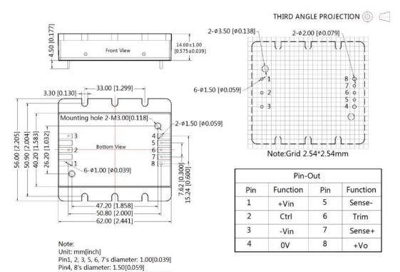
Pin diameter tolerances: ±0.10[±0.004] General tolerances: ±0.50[±0.020] Mounting hole screwing torque: Max 0.4 N·m
