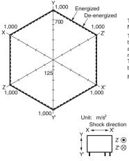
Test Item: G5NB-1A-E, 24VDC Number of Relays: 5 pcs Test Method: Shock is applied 3 times in 6 directions along 3 axes
