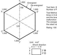
Test Item: G5NB-1A, 24VDC Number of Relays: 5 pcs Test Method: Shock is applied 3 times in 6 directions along 3 axes and the level at which shock caused malfunction is measured. The energized voltage is 100% of the rated voltage. Rating: 100 m/s<sup>2</sup>
