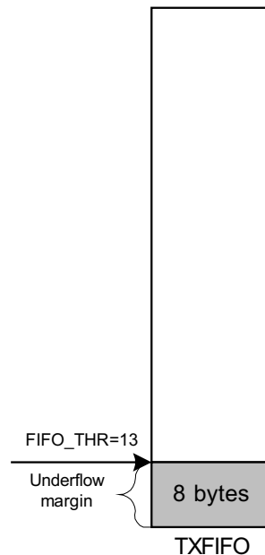
Figure 5-14. Example of FIFO at Threshold
