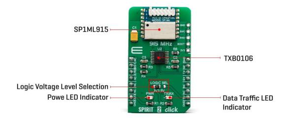
The primary function of the SP1ML-915 module is to be used as a wireless serial cable replacement. The Click board<sup>™</sup> features the SWD compatible programming header, allowing custom firmware to be uploaded to the integrated MCU. However, that may destroy the factory firmware and void the warranty.
