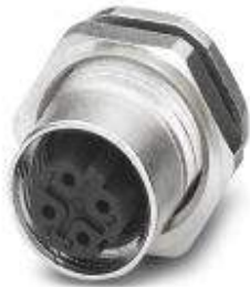
Bus system flush-type socket, ETHERNET, 4-pos., M12 SPEEDCON, D-coded, rear/screw mounting with PG9 thread, with straight solder connection
