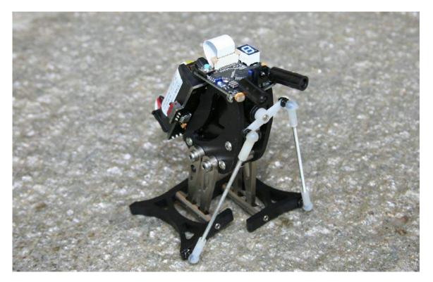
The Penguin's microcontroller is an embedded BASIC Stamp2px24 module, the fastest and most powerful BASIC Stamp microcontroller model in the Parallax lineup. The Penguin requires three hours to assemble, after which it is a PBASIC programming challenge to exploit all of the robot's capabilities.
