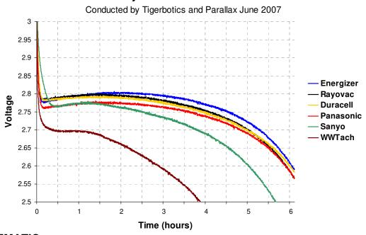
CR123 Battery Test with 200 mA Current Draw
