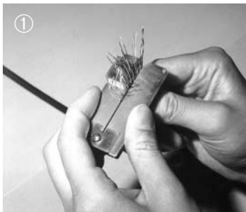
1. Set the wires in the wiring fixtures.
