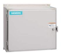
2-speed 3-phase motor starter, Size 0, One winding consequent pole, Constant or variable torque, Solid-state overload relays, Low Spd OLR range 0.75-3.4A, High Spd OLR range 0.75-3.4A, 110V 50Hz / 120V 60Hz coil, Enclosure NEMA type 12, Dust/drip proof for indoors
