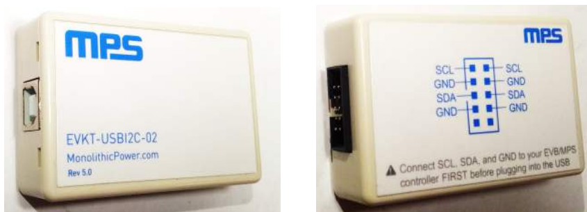
Figure 4: USB-to-I 2 C Communication Kit
