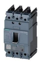
circuit breaker 3VA5 UL frame 125 breaking capacity class H 65kA @ 480V 3-pole, line protection TM230, FTAM, In=90A overload protection Ir=90A fixed short-circuit protection Ii=5...10 x In UL 489 SB (naval), 50° C without connection
