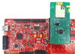
Fig 4: Programming and debugging with CY8CKIT-042-BLE BLE Pioneer Kit Baseboard
