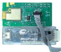
Fig 3: Programming/Debugging with MiniProg3
