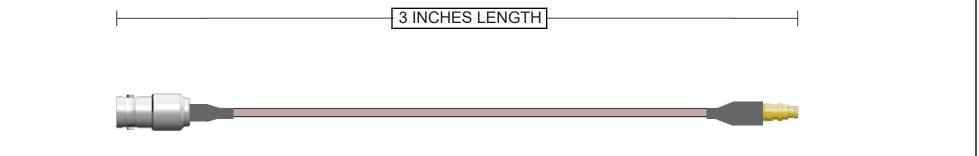
Connector A 112631 BNC Jack Straight Brass Nickel + Heatshrink 50 Ohm RG-178 Continuity/Hi-Pot Connector B 925-129C-51S SMPM Plug Straight Brass Gold + Heatshrink
