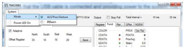
By default, the GUI is set for ALS/PROX/Gesture memory space/mode. While in this mode, IRBeam cannot be evaluated because the shared device memory space is controlling gesture functions. If IRBeam is to be evaluated, then the user must select IRBeam from the "System" menu as shown above. It is possible to switch between IRBeam and ALS/Prox/Gesture, but care must be taken to manually set (reset) the "Enable" bits (address 0x80) each time a switch is made.
