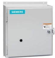
Mechanically held lighting contactor, Contactor amp rating 100Amp 0NC  $\_$  3NO poles, 220VAC 50HZ / 240VAC 60HZ coil Non-combination type, Enclosure NEMA type 12, Dust/drip proof for indoors
